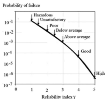
Fig. 3. USACE (1997) guidelines for reliability index and the corresponding probability of failure [10]
