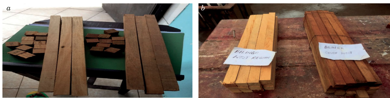
Fig. 1. Sample piece: (a) raw material, (b) prepared sample for mechanical characterization
